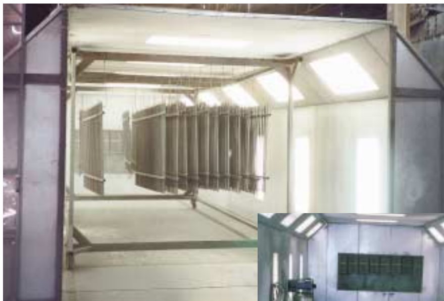
The shop made its three batch coating booths for handling parts more than 40 feet long.
